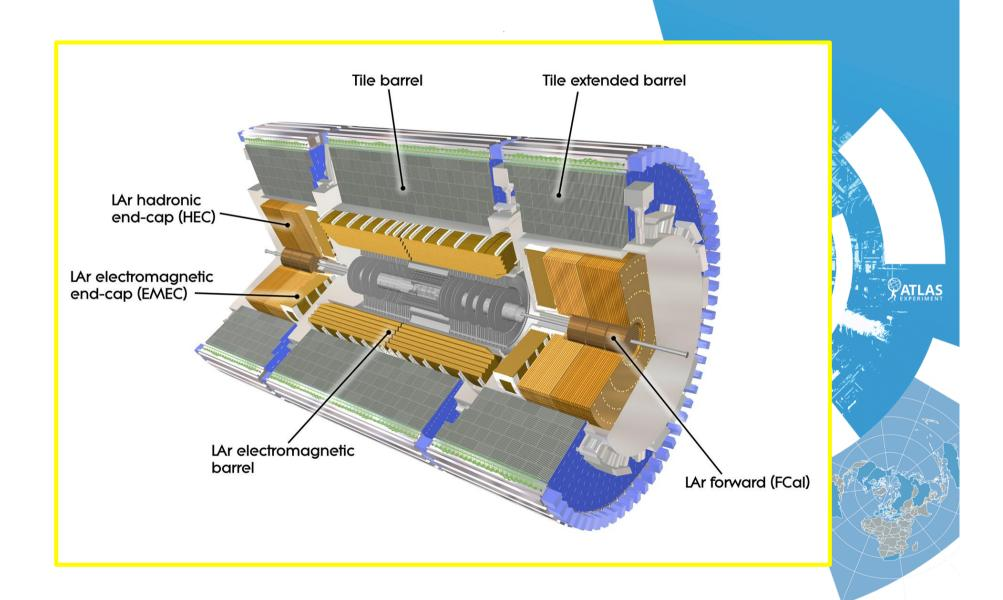
The Liquid Argon (LAr) Calorimeter works with Liquid Argon at -183 degrees C
